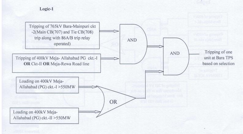
Note- To avoid the loading on 400kV Meja- Allahabad PG ckt.-I &II to go beyond 650 MW following the tripping of 765 kV Bara-Mainpuri Ckt –II ,as a Standard Operating Procedure, control room operator shall take action to bring down generation at Bara TPS to restrict the loading on 400kV Meja- Allahabad PG ckt.-I &II below 550 MW
