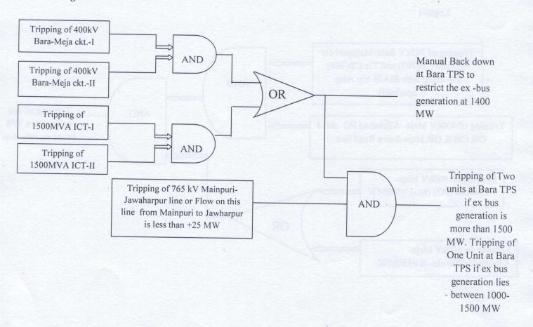
Note- As a SOP, Bara TPS shall ensure that selection of Unit for tripping is done in such a way that Unit with highest generation gets tripped.
