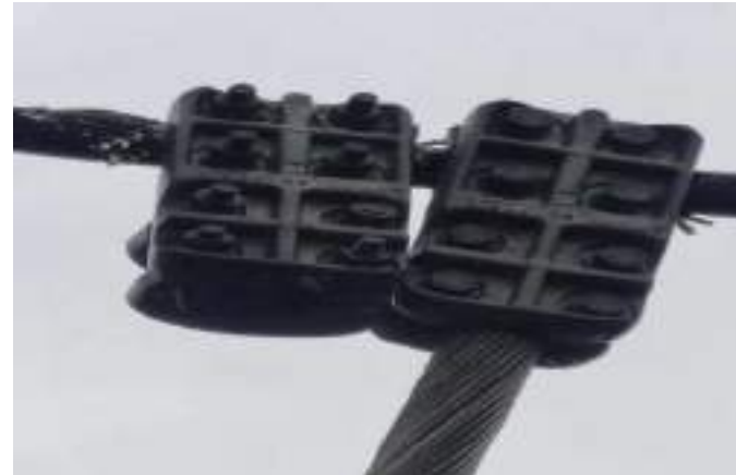
Damaged conductors at dead end and CVT jumper
